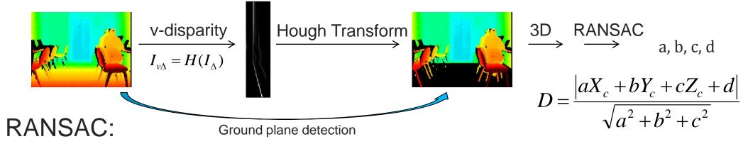
The offline phase of the algorithm utilizes RANSAC [Fischler, 1981] for plane coefficients calculation.
